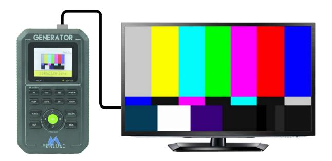
How to Test a Sink (a sink is anywhere the signal ends up such as a TV, Projector, or Computer Monitor)
