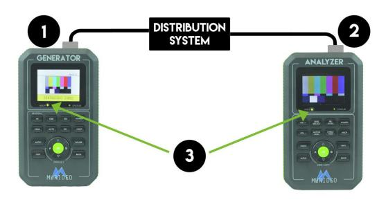
In the system diagram above it's easy to see the basic components of a video distribution system. Obviously, this is a very simple system diagram, use your imagination to replace all the sources, displays, matrices, distribution amplifiers and extenders in the system [where you see the term – DISTRIBUTION SYSTEM above] and the task of troubleshooting these systems can become daunting at times.
